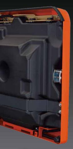
Three mud-cleaning ports ensure fast and simple removal of mud and debris from the lower part of the machine.
